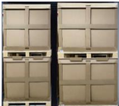
Replaced plastic straps with paper straps.
